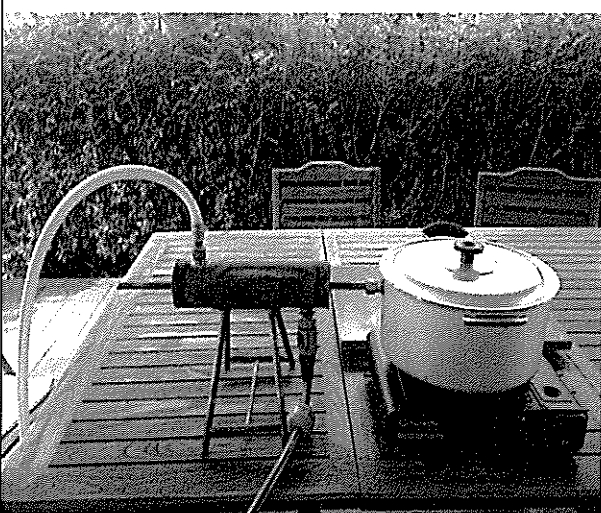
Test run of the components by using water to see whether the cooling chamber works
